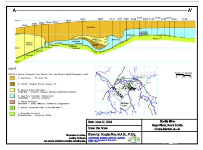
Figure 7-11: Geological Cross-Section A-A'
