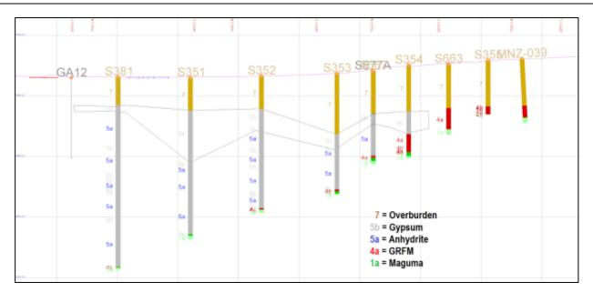
Figure 14-2: Section View of Gypsum Domain
