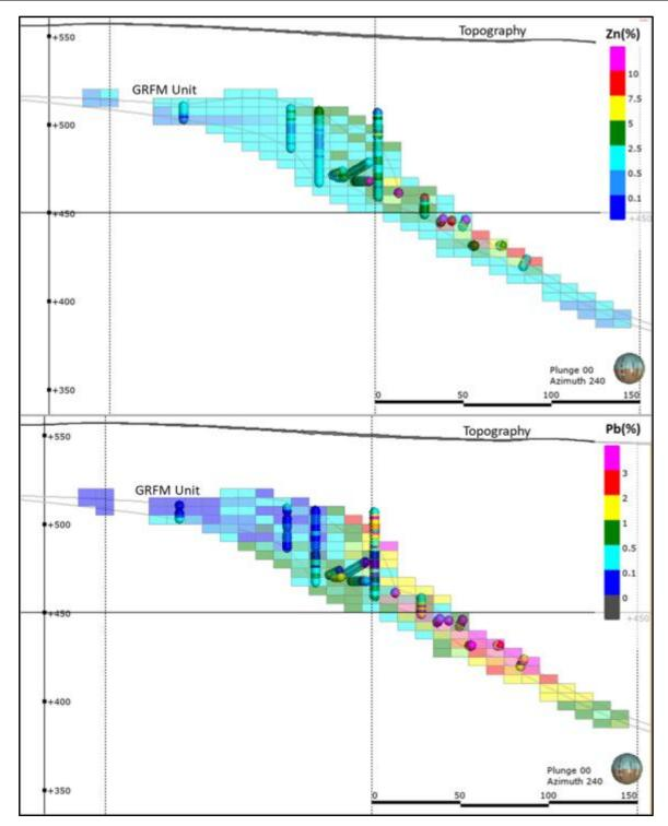
Figure 14-9: Main Zone Cross-Section Comparing Assay Composite Grades to Estimated Block Grades for Both Zn and Pb (Section Looking South-West)
