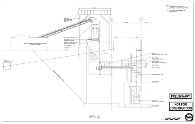
Figure 17-4: Crushing Area Section
