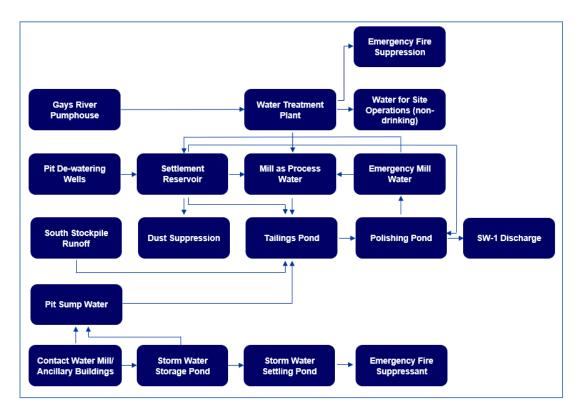
Figure 20-5: Scotia Mine Water Process Flow Chart
