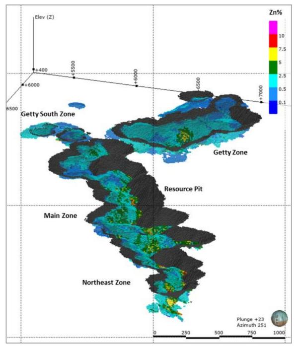
Figure 14-16: 3D Isometric View of the Resource Pit and Block Model (Zn% Grade Shown) Source: SRK 2019
