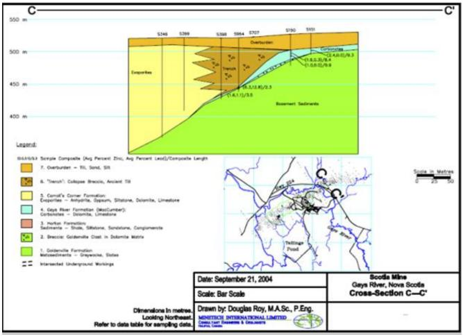
Figure 7-13: Geological Cross-Section C-C'
