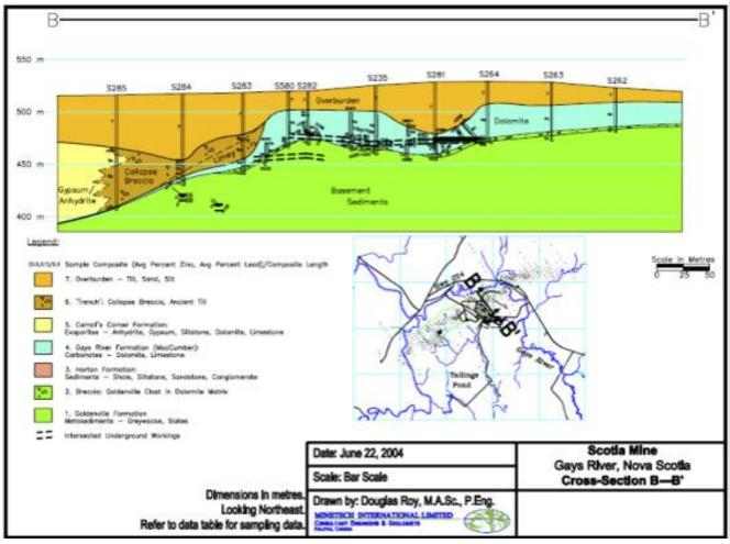
Figure 7-12: Geological Cross-Section B-B'
