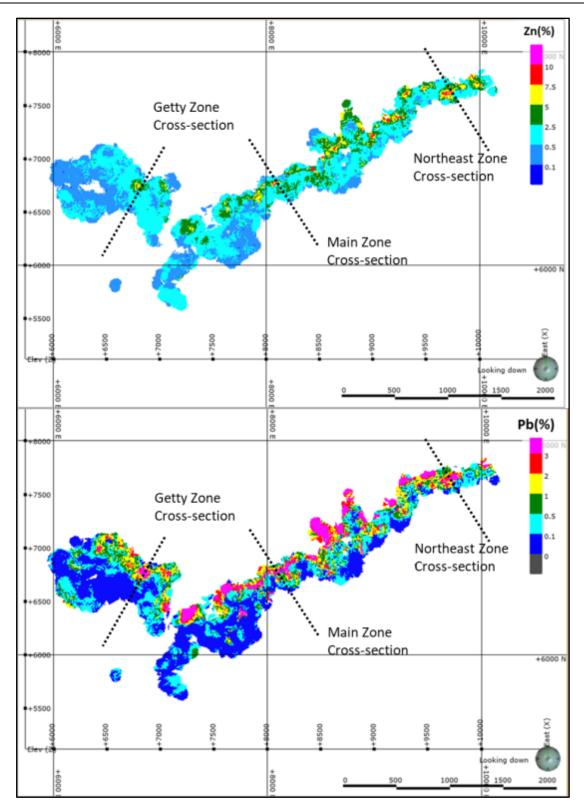
Figure 14-8: Plan View of Zn and Pb Block Grades and Cross-Section Locations for Main, Getty and Northeast Zones
