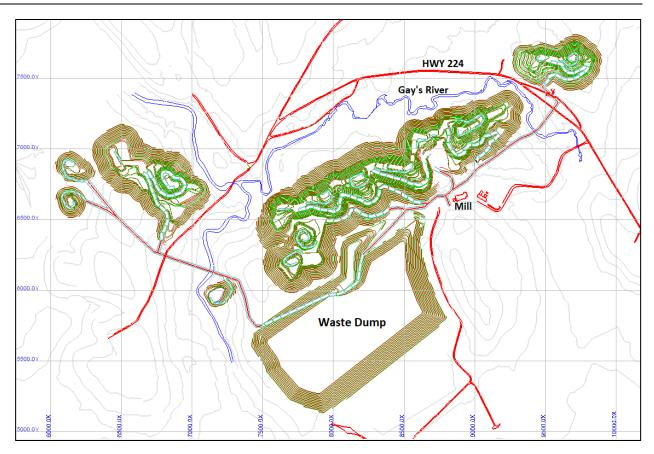
Figure 18-61: Waste Rock Storage: Waste Dump Design
