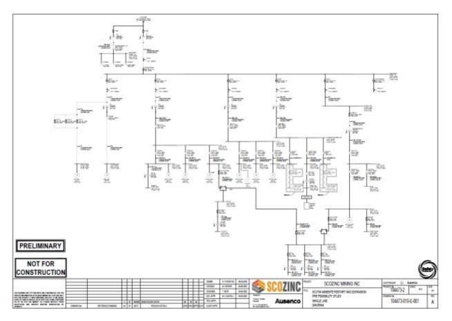
Figure 18-6: Existing Electrical System Single-Line Diagrams
