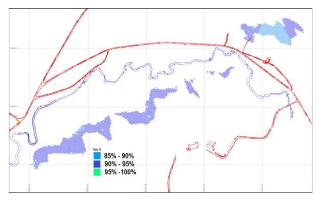
Figure 14-12: Plan View of Gypsum Block Grades
