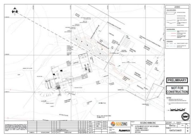
Figure 18-34: Proposed Additions to Mill Process Building
