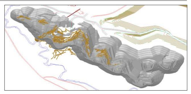
Figure 16-27: 3D View of Underground Workings Network Within the Main Zone Pit
