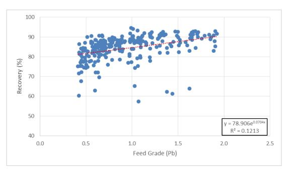
Figure 13-3: Lead Recovery Model for Cash Flow Analysis
