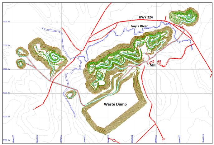
Figure 16-18: Ultimate Pit Design & Dump Design
