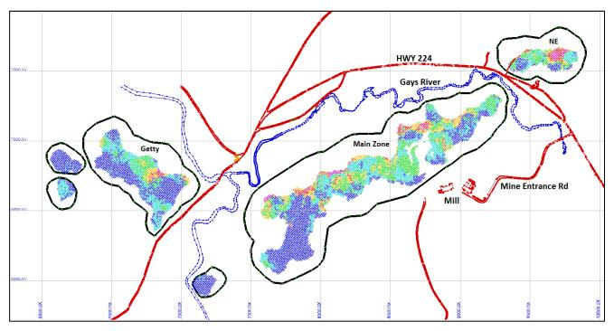
Figure 15-2: Orebody with Surface Constraints
