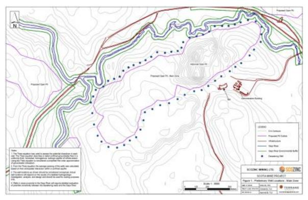
Figure 16-28: Overburden Slope Depressurizing Well Locations
