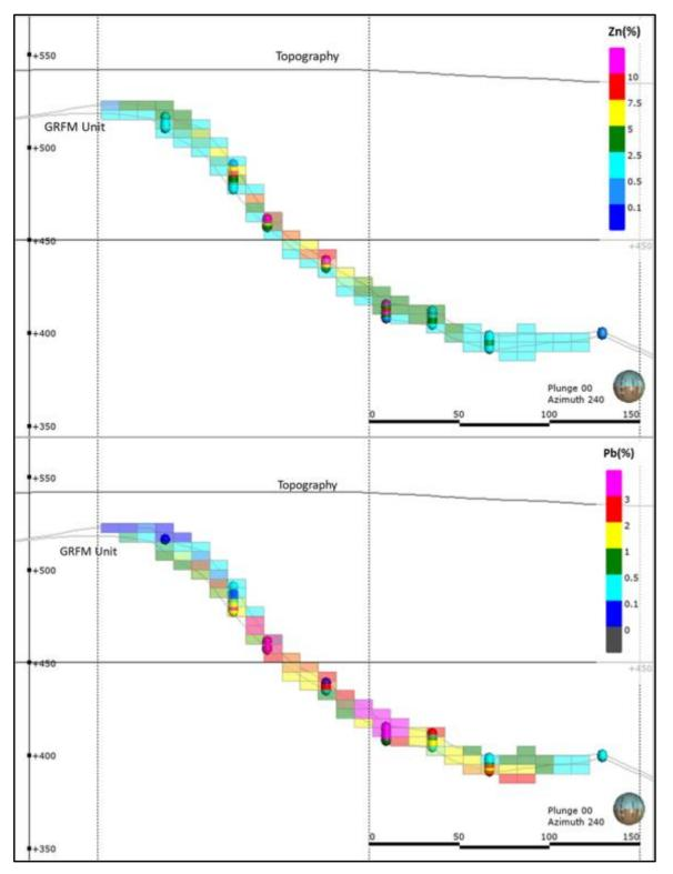
Figure 14-11: Northeast Zone Cross-Section Comparing Assay Composite Grades to Estimated Block Grades for Both Zn and Pb (Section Looking South-West)
